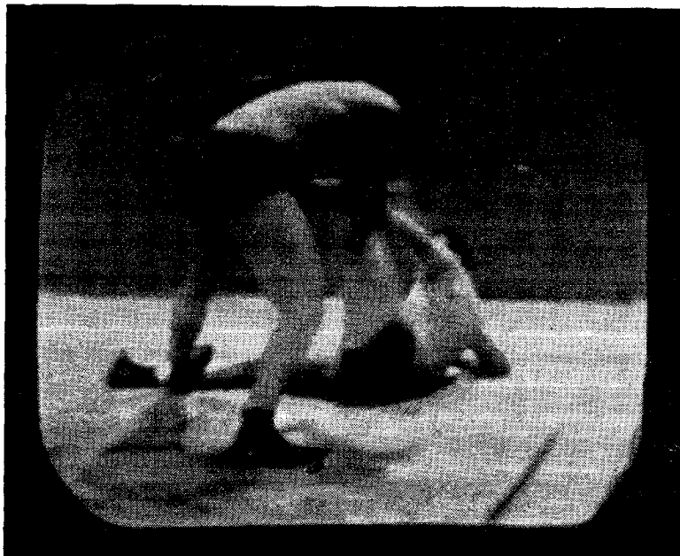
The growth of television is closely linked with abatement of the interference nuisance. This un-retouched photograph hardly gives an adequate idea of the "annoyance value" of motor ignition interference (note the white spots).
